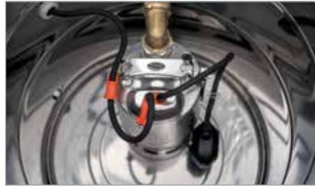
Submersible stainless steel pump for oil discharge
