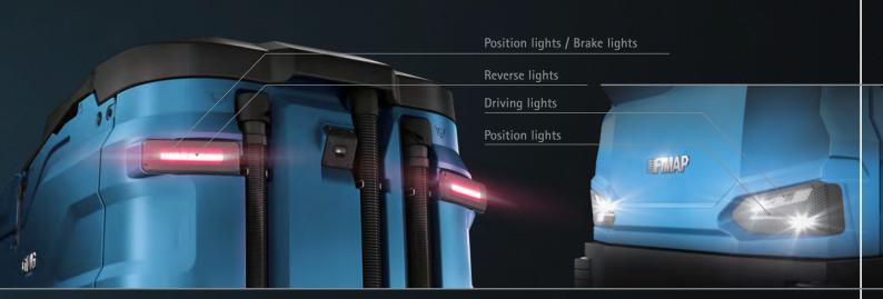
PASSIVE SYSTEMS to help the operator in case of emergency
