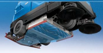
DUAL DISC with 2 disc brushes or 2 pad holders **CYLINDRICAL** with 2 cylindrical brushes and a debris hopper for small sized solid debris
