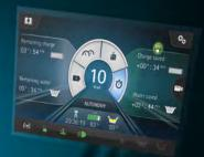
remaining autonomy of batteries and tank, and projection of savings that can be achieved in Eco Mode
